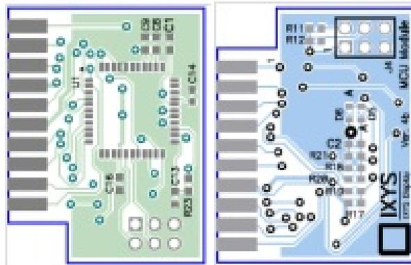
**Figure 13: Layout of Digital Control Module –Top and Bottom Layers (Not to Scale)**
