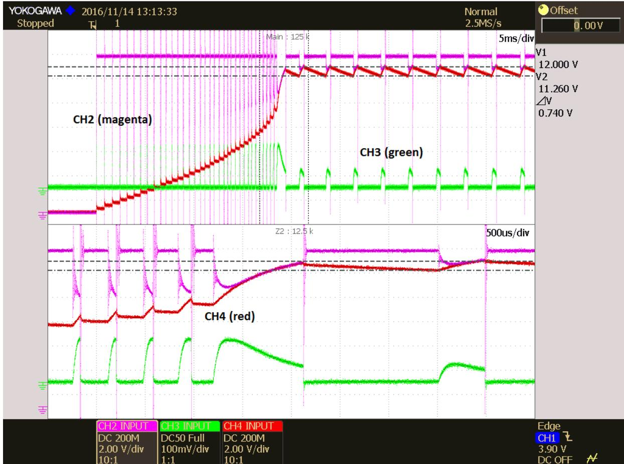
**Legend:** Channel 2 (magenta) – battery voltage, Channel 3 (green) battery current, Channel 4 (red) – output voltage
