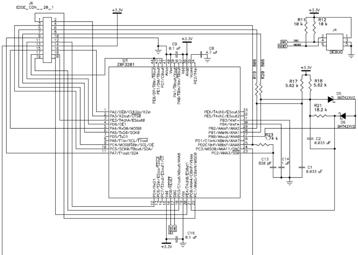
**Figure 3: MCU Board Circuit Schematic Diagram**
