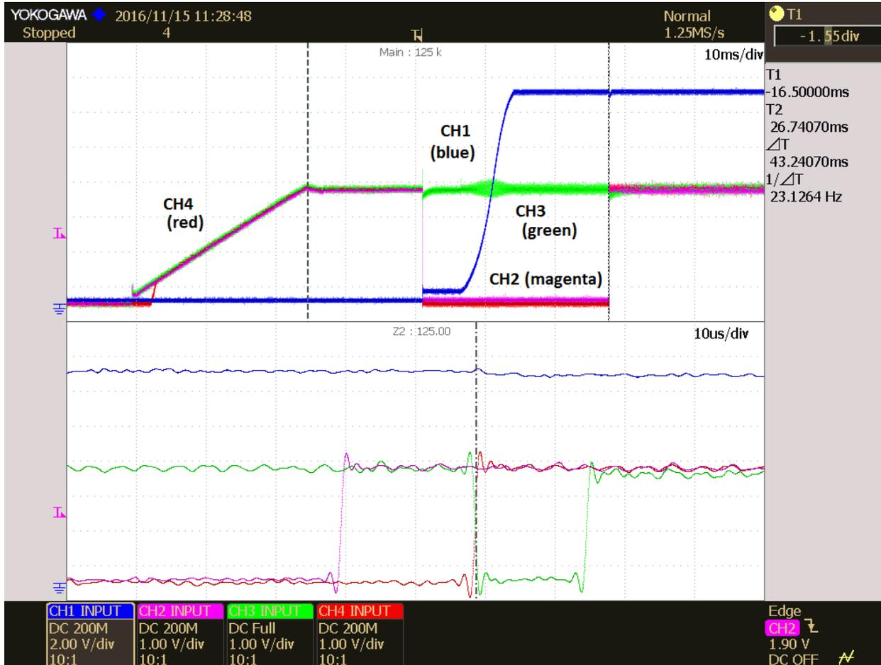
**Legend:** Channel 1 (blue) secondary side voltage, Channel 2 (magenta) – trigger U3 “reset” signal
