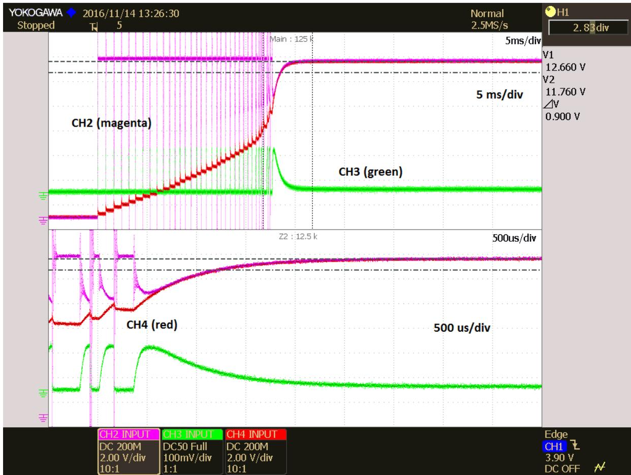
**Legend:** Channel 2 (magenta) – battery voltage, Channel 3 (magenta) battery current, Channel 4 (red) – output voltage
