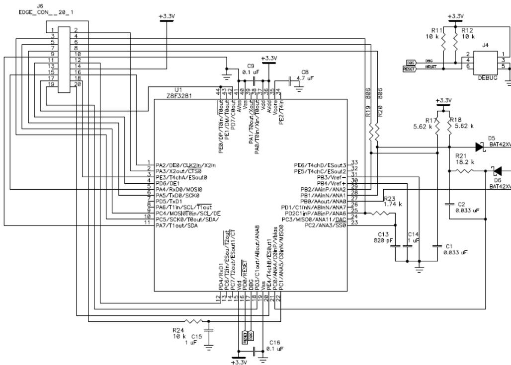
Figure 12: Schematic Diagram of Digital Control module
