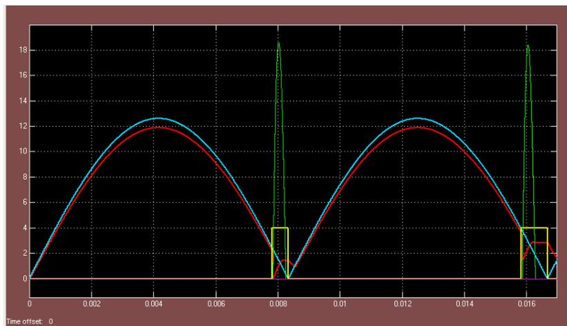
Figure 3: Capacitor C pre-charging during first 2 cycles. Legend: Blue – power line voltage, Red - voltage on Capacitor C in respect to common Ground, Yellow – driver to Sw1, Green – Capacitor current. (Not to scale)
