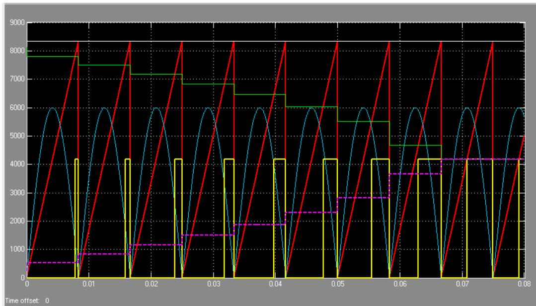
Figure 4:  $T_{on}$  timing generation. Legend: Blue – rectified power line voltage, Red – full cycle period timing counter, Yellow – driver to Sw1, Green – time OFF to Sw1, Magenta – Time ON to Sw1, White – period T.
