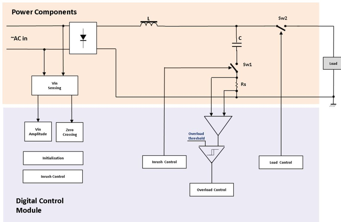
Figure 1: Functional Block Diagram of the Digital Inrush Controller
