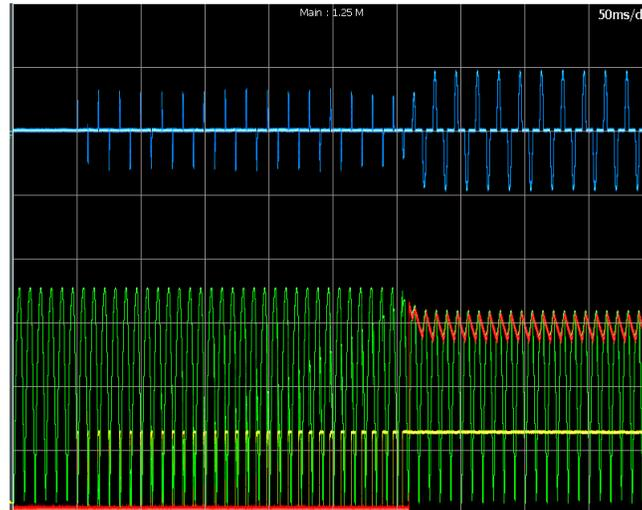
Figure 9: Scope snapshot of inrush pulses with N increased to 16. Legend: Blue – power line current (10A/div), Red – Load voltage (50V/div), Green – rectified input voltage (50V/div), Yellow – driver to Sw1.
