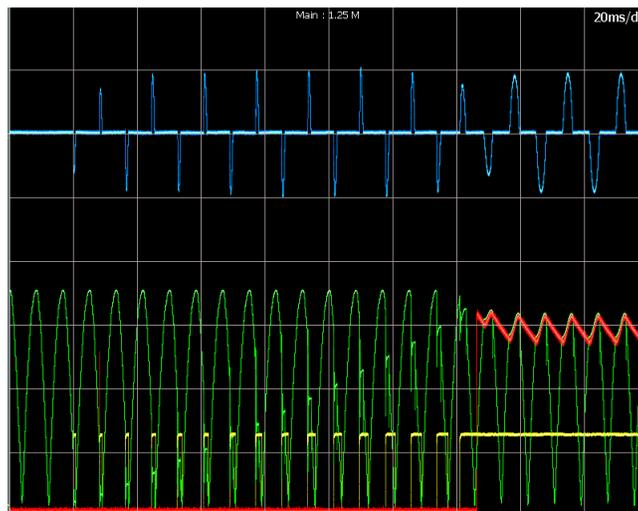
Figure 8: Scope snapshot of the Digital Inrush Current Control. Legend: Blue – power line current (10A/div), Red – Load voltage (50V/div), Green – rectified input voltage (50V/div), Yellow – Sw1 commutation signal.
