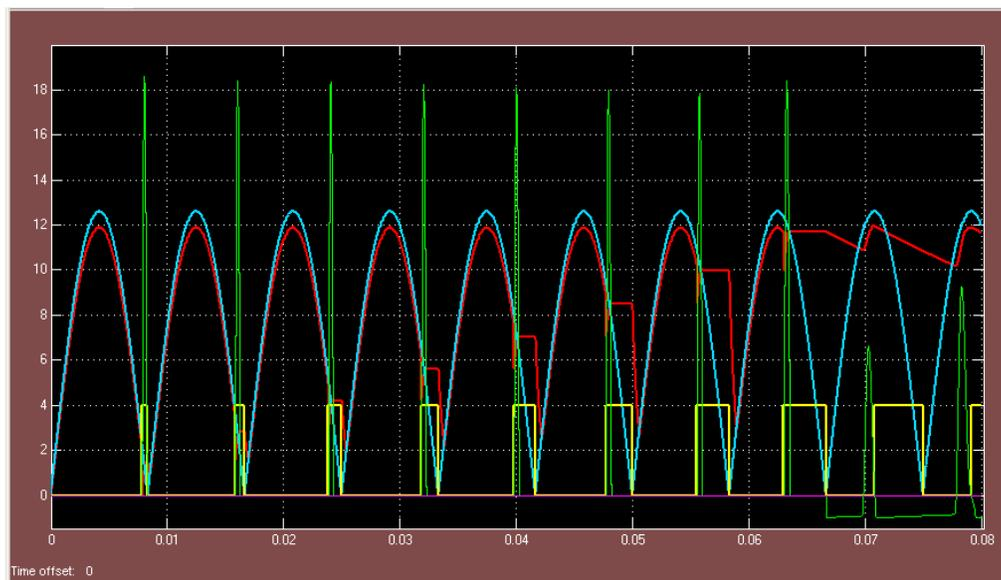
Figure 5: Capacitor C pre-charging. Legend: Blue – rectified power line voltage, Red – voltage Capacitor C in respect to common Ground, Yellow – driver to Sw1, Green – Capacitor current.
