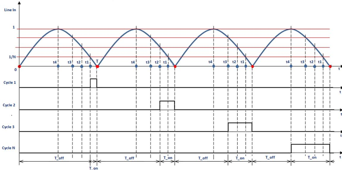
Figure 2: Digital Inrush Control timing
