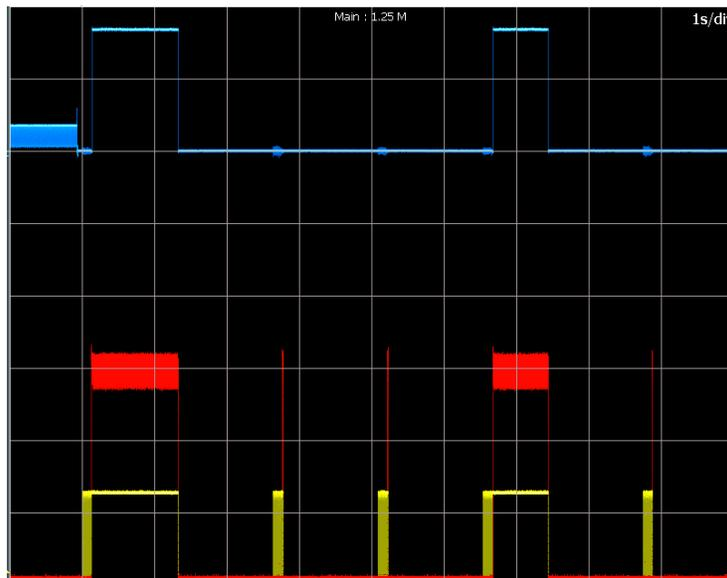
Figure 10: Scope snapshot to illustrate Overload and restart. Legend: Blue –Power Good status, Red – Load voltage (50V/div), Yellow – driver to Sw1.
