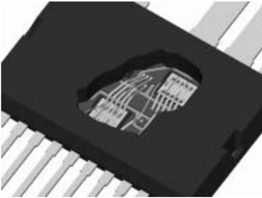
Figure 6: enlarged cut-off view of proposed GWM160-0055P3 component
