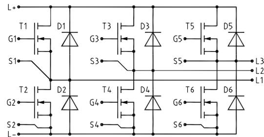
Figure 1: MOSFET three phase full bridge
