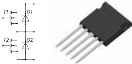
Figure 3: MOSFET phaseleg: symbol and external view of isolated ISOPLUS i4™ package  $21mm \cdot 20mm \cdot 5mm$
