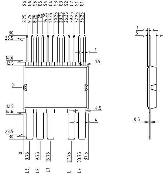
Figure 5: pinout and dimensions of proposed GWM160-0055P3 component
